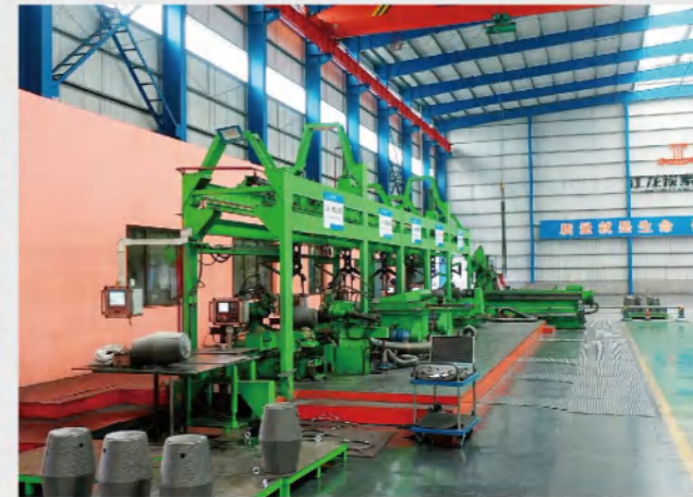
全自动石墨电极接头机加工系统 Fully Automatic Graphite Electrode Nipple Machining System
