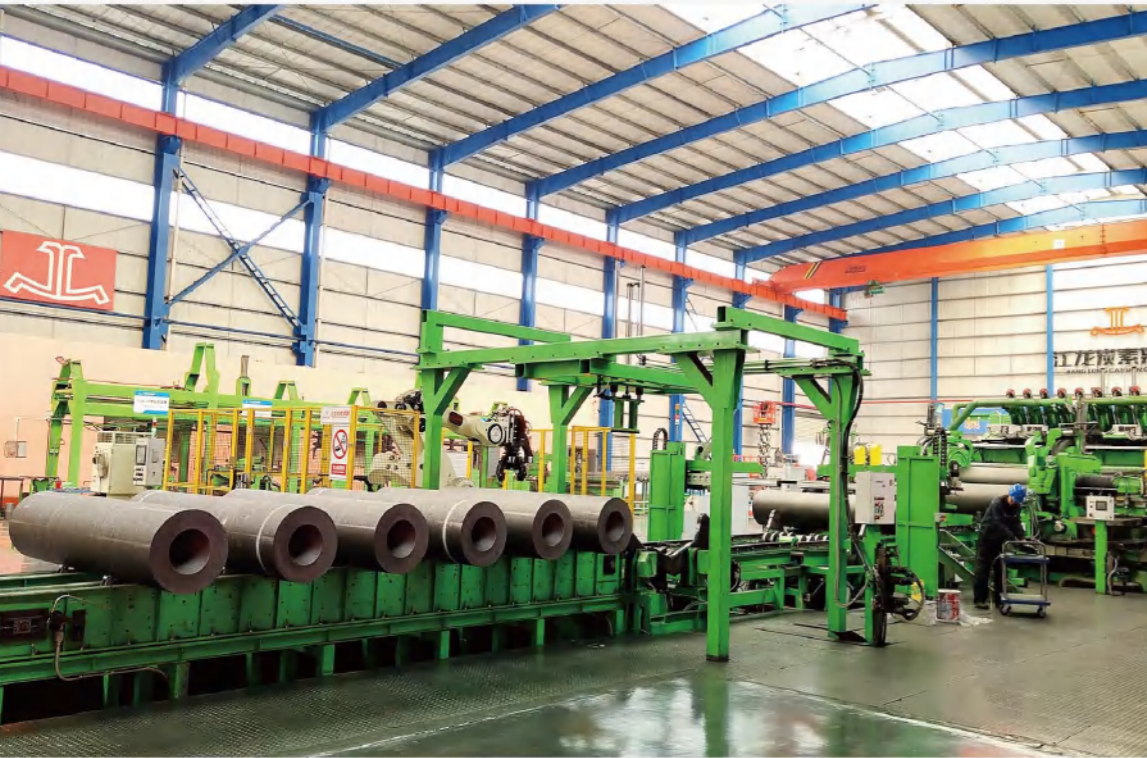
日本进口NACHI全自动石墨电极本体机加工系统 Fully Automatic Graphite Electrode Machining System Imported From NACHI Japan
