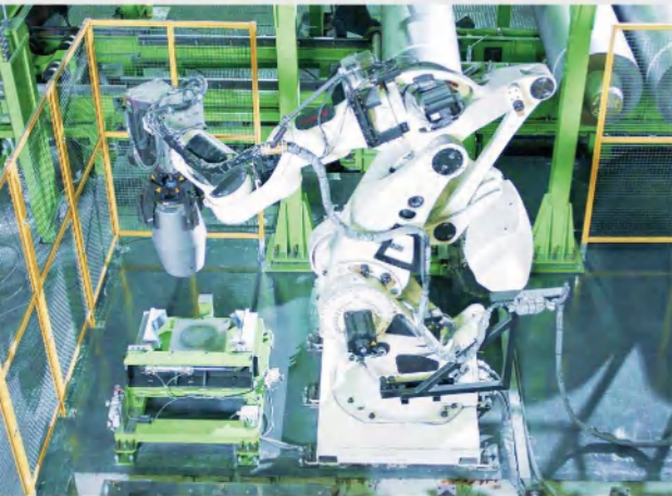
日本进口NACHI石墨电极接头预组装系统 Graphite Electrode Nipple Pre-assembly System Imported from NACHI Japan
